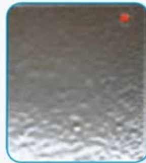
Fig 2 After 10 minutes in vertical position, 100% of AZO™ GEL remains on the surface of the test plate
